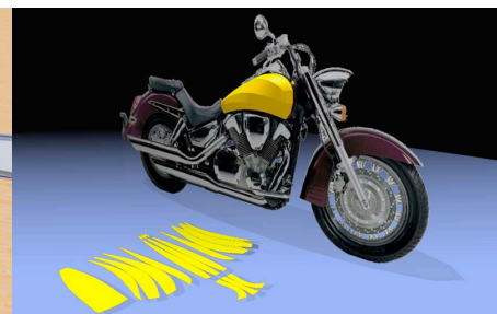
Sheet metal. TouchCAD comes with many build in tools for sheet metal objects such as cones, T-joints, etc. Such objects can be modified in any way, and it is also possible to generate free-form sheet metal objects and unfold them.
