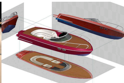
Reverse engineer 3D models by means of high resolution background images. Imported images can be corrected in scale, rotation, proportions, perspective, and be place them correctly relative to other images.
